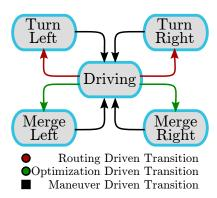
Fig. 2. **Finite State Machine:** We highlight different behavior states that are determined by the routing and optimization algorithms. When executing turns, the routing algorithm transitions the behavior state to a turning state. When the optimization-based maneuver algorithm plans a lane change, the behavior state is transitioned to merging.
