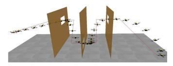
Fig. 1. The *3-Window* scenario for our quadrotor simulation experiments. The red line is the guiding path. Our approach smoothly controls the quadrotor (shown at 4Hz) through the windows without colliding with the walls. Videos are available at http://gamma.cs.unc.edu/CA/LQGObs/.
