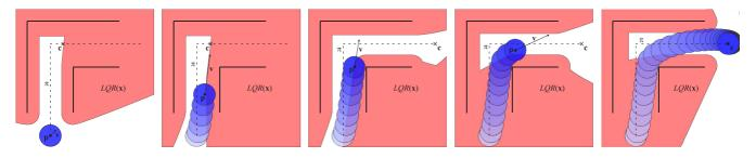
Fig. 3. Navigating a circular robot whose acceleration can be controlled (see Section V-B) through a narrow corridor using LQR-Obstacles. The workspace obstacles are shown using thick lines. The guiding path  $\pi$  is shown by a dashed line. In each frame, the LQR-Obstacle  $\mathcal{LQR}(\mathbf{x})$  for the particular state  $\mathbf{x} = (\mathbf{p}, \mathbf{v})$  is shown. The valid configuration  $\mathbf{c}$  farthest along the guiding path is chosen as target configuration.
