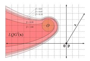
Fig. 4. The LQG-Obstacle  $\mathcal{LQG}^{\bar{p}}(\hat{\mathbf{x}})$  in the same configuration as in Fig. 2 accounting for motion and sensing uncertainty of the robot (see Section V-B). The conservative approximation of Eq. (25) is shown for various values of the probability bound  $\bar{p}$ . For  $\bar{p} = 1$ , it is equivalent to the LQR-Obstacle.
