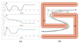
Fig. 8. (a) The x, y, and z position over time of the quadrotor in the *3-Window* scenario (see Fig. 1). (b) The xy-projections of the maximum likelihood traces of the quadrotor in the *S-Maze* scenario (see Fig. 7) for 0, 1, 2, and  $5 \times$  the realistic amount of uncertainty.
