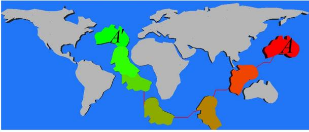
Fig. 4. *World Map Example: This figure shows an application of our C-obstacle query to speed up a complete motion planner - the star-shaped roadmap method. In this example, the object needs to move from initial configuration A to goal configuration A' by translating and rotating within the shaded rectangular 2D region. Our C-obstacle query can achieve about 2.0 times speedup for this example.*
