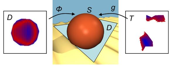
**Figure 4: Texture-Based Collision Detection Process.** Center: A sphere  $S$  collides with a textured terrain. Left: Contact plane  $D$  for texture-based collision detection, and mapping  $\phi : D \rightarrow S$ . The contact plane shows the penetration depth. Right: Dynamic deformation texture  $T$ , and mapping  $g : T \rightarrow S$ . The penetration depth is projected from  $D$  to  $T$ , and is available for collision response.
