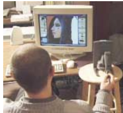
Figure 3: Haptic Painting System Setup: An artist using a haptic stylus to paint directly on the virtual canvas using DAB.
