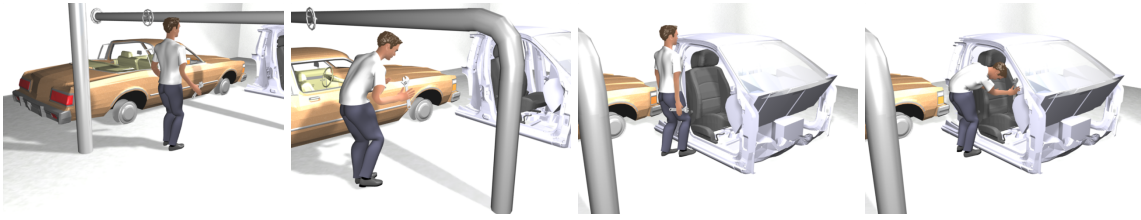
Figure 5: Walking-and-Bending: The human model walks towards the car, avoiding some obstacles. It bends and stretches to put the tool inside the car. The latter is a highly constrained environment and we need to perform whole-body planning to generate such motions.
