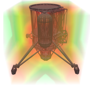
Figure 7: Cassini Model: A volume rendering of the distance field of the Cassini with 93K polygons. The distance to the surface is color coded, increasing from red to green to blue.
