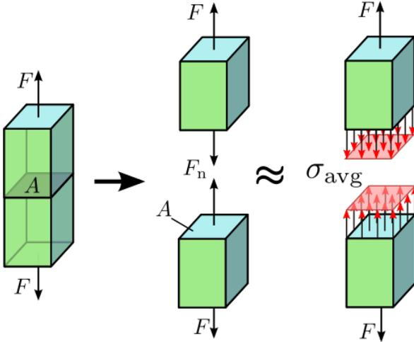
Fig. 1: The figure shows force vector normal to the surface or parallel to the surface. Copyright Wikipedia [2]
