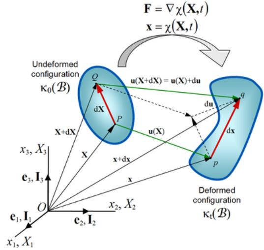
Fig. 5: The figure shows the displacement field and the deformation gradient. Copyright Wikipedia [5]
