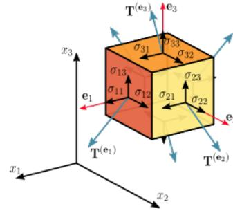
Fig. 2: The figure shows the components of the cauchy stress tensor. Copyright Wikipedia [2]
