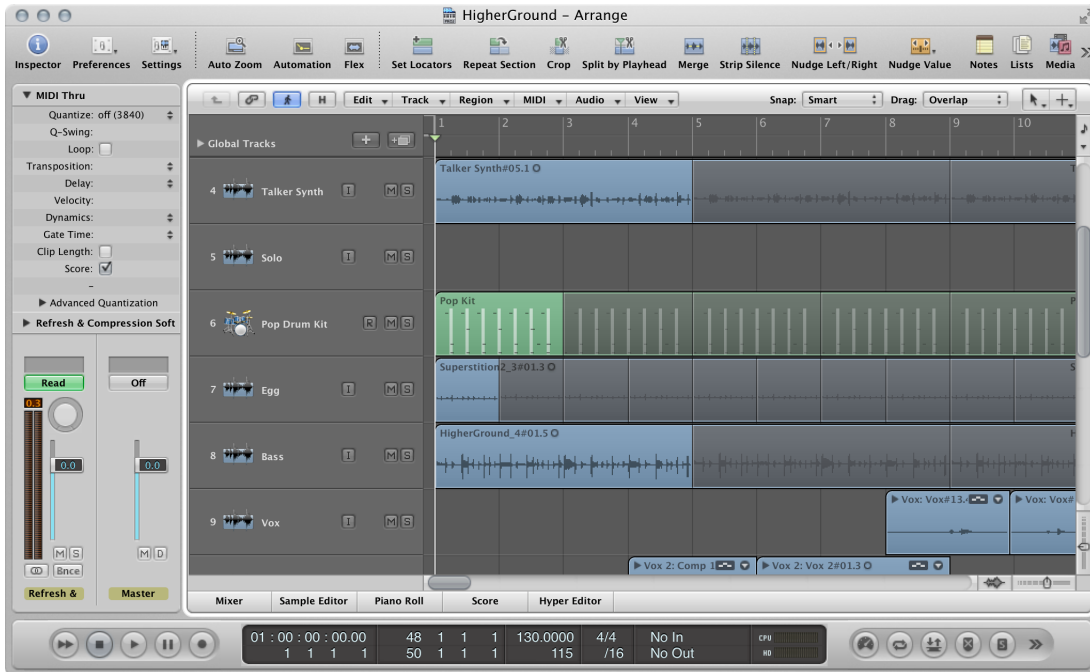
Figure 1: Apple’s Logic Pro DAW’s main view uses a common timeline layout, with individual audio tracks, each containing audio clips arranged in time, layered together to produce the composite output. Effects are applied on a per-track basis using plugins (not pictured) and affect any audio clips on a track’s timeline.
