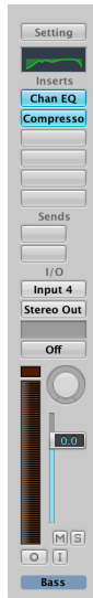
Figure 2: Plugins get added to individual channel strips in series. This channel's audio gets sent through an equalization plugin (for frequency manipulation) then a compressor plugin (to limit dynamic range).
