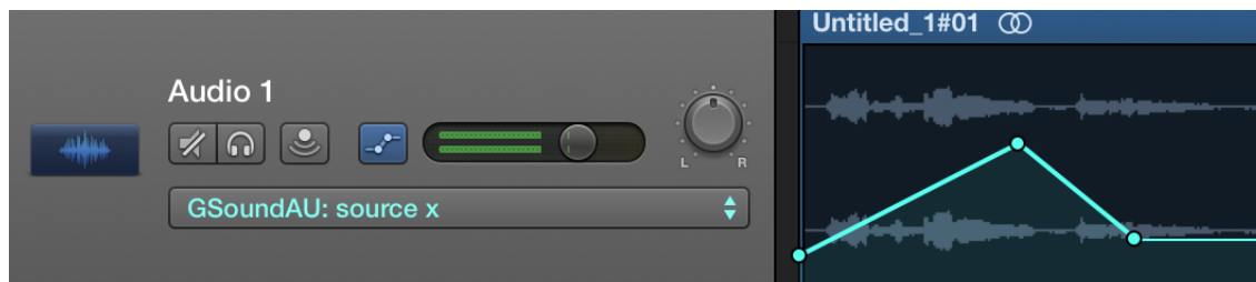
Figure 4: Full integration with DAW hosts allows users to animate GSoundAU parameters (such as the x coordinate of the source position) in the main timeline window.
