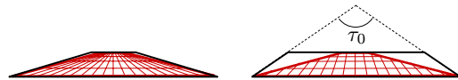
Figure 11: \tau -Limiting. (Left) a face partition with excessive shearing caused by a large angle \tau between the edges of the trapezoidal region to which to parameterization is applied (black). (Right) Limiting \tau to some constant \tau_0 reduces the shearing at the expense of error at the narrow end of the face partition.
