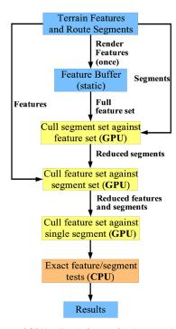
We use three forms of GPU culling before performing exact intersection tests between features and segments.
