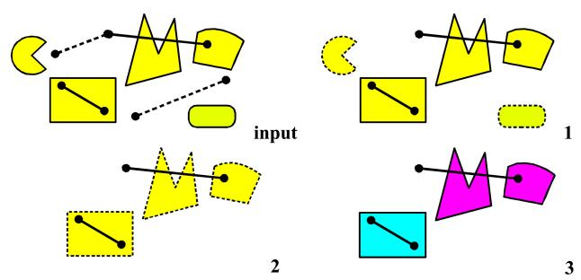
Our GPU-based culling algorithm proceeds in three phases. First, non-intersecting segments are pruned. Second, non-intersecting features are pruned. Third, potentially intersecting features are paired with segments.
