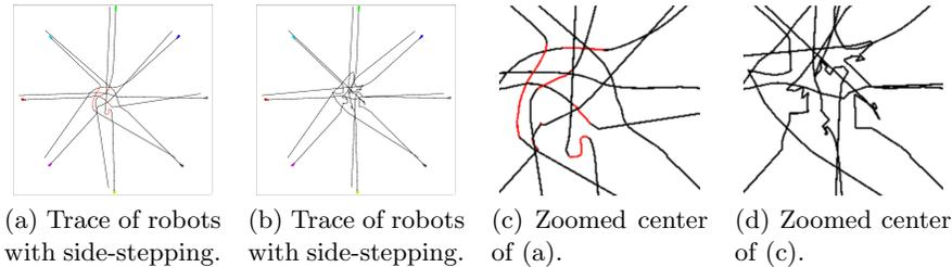
Fig. 5: Comparison of computed trajectories of *Circle* benchmark with and without side-stepping. Black segments show the forward walking motions, and the red segments show side-stepping motions.
