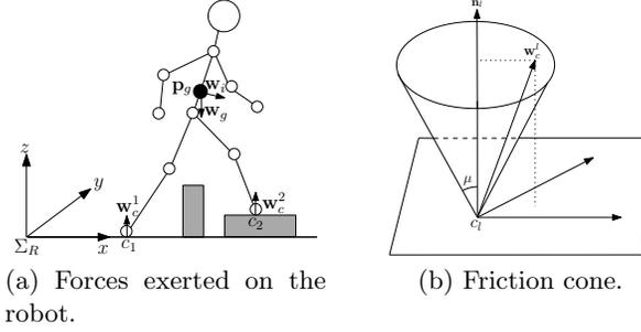
Fig. 3: A human-like robot makes contacts  $c_1$  and  $c_2$  with the ground plane. The gravity force  $\mathbf{w}_g$  and the inertia force  $\mathbf{w}_i$  are applied to the robot. The contact forces  $\mathbf{w}_c^1$  and  $\mathbf{w}_c^2$  can have values in their friction cone. The robot is stable when  $\mathbf{w}_c^1 + \mathbf{w}_c^2 + \mathbf{w}_g + \mathbf{w}_i = \mathbf{0}$ .
