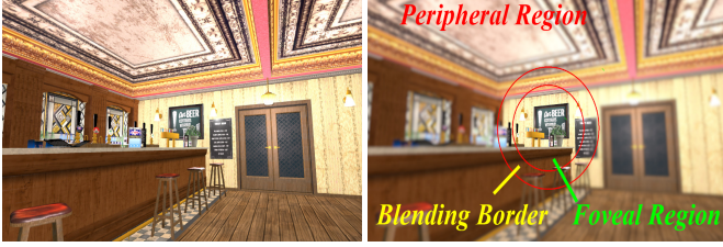
Fig. 8: Application of our gaze prediction to gaze-contingent rendering. Left: Rendered in normal mode; Right: Rendered using gaze-contingent rendering mode. Gaze-contingent rendering decreases rendering quality in the peripheral region while maintaining high fidelity in the foveal region. The inner circle is the foveal region rendered with high quality, the outer region is the peripheral region rendered with low quality and the blending border denotes the transitional region.
