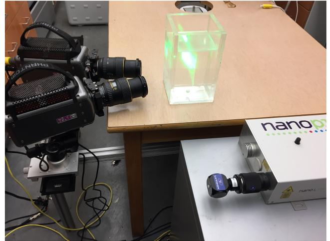
Fig. 1. Our PIV setup to capture velocity fields. Laser is injected into viscous fluids to capture the 2D velocity fields on the sheet.
