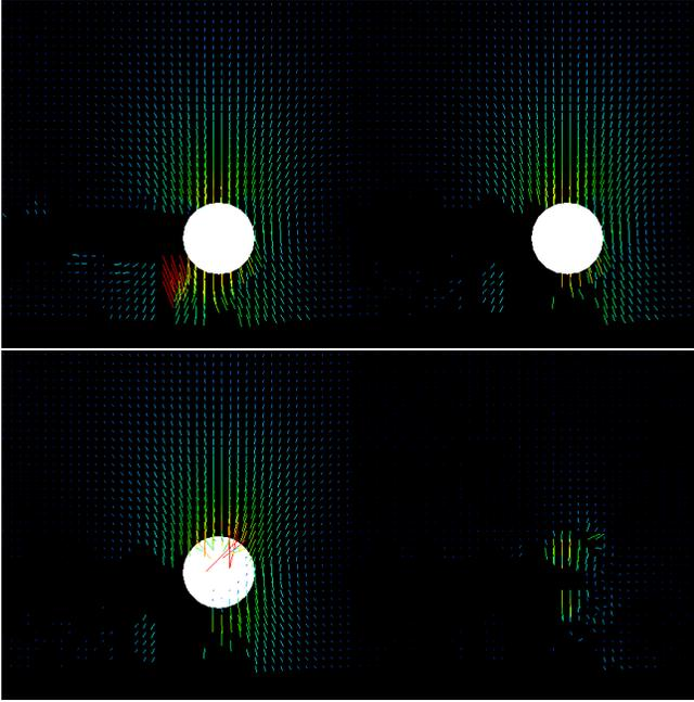
Fig. 2. Velocity field illustration. White sphere represents the solid ball falling inside the viscous fluids. (Top left) velocity fields captured with PIV. (Top right) valid velocity fields. (Bottom left) velocity fields interpolated from velocity fields generated with our solver. (Bottom right) Velocity field differences between the valid velocity fields and the interpolated velocity fields.
