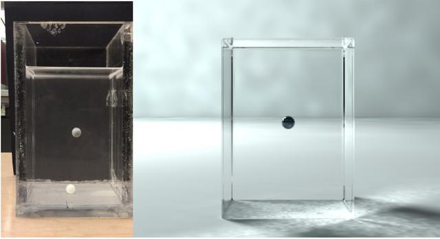
Fig. 3. A sphere falling inside of viscous fluids. (Left) experimental setup for capturing PIV velocity fields. (Right) our simulation results with the identified viscosity parameter. The falling behavior of the simulated ball is in good agreement with the falling ball in the real world used to capture PIV data.
