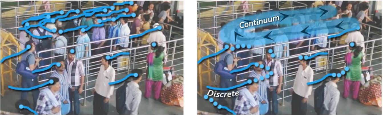
Fig. 2: The left image highlights the tracked trajectories based on discrete motion models. The image on the right demonstrates the use of a hybrid motion model, using the continuum method for a cluster of pedestrians as well as discrete motion models for individuals. These clusters are computed in realtime based on frame coherence and pedestrian flow. The hybrid motion model can improve the tracking accuracy in these dense scenarios by 7-12% over prior methods.
