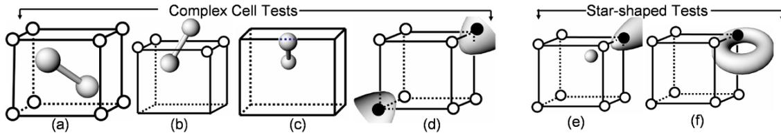
**Figure 2:** This figure shows the different cases corresponding to the complex cell and star-shaped test. Figs (a), (b), (c) and (d) show cases of complex voxel, complex face, complex edge, and topological ambiguity. The white and black circles denote positive and negative grid points respectively. Fig. (e) shows the case where the surface is not star-shaped w.r.t a voxel. In Fig (f), the restriction of the surface to the right face of the cell is not star-shaped.
