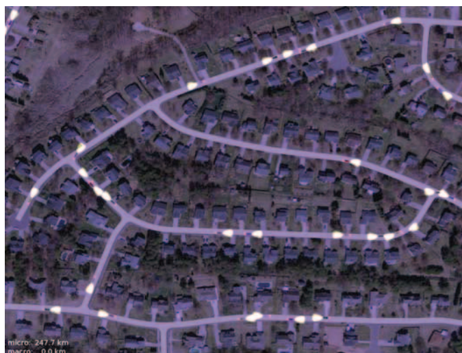
Fig. 1. A road network generated directly from GIS data by our method. The road network has been overlaid on top of a satellite image. Note that the cars on the road network are animated using a traffic simulator running on our road network representation.
