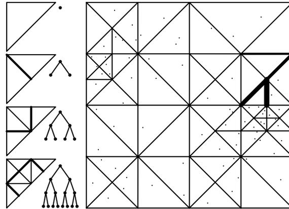
**Figure 1:** A binary triangle tree (BTT) hierarchy is illustrated (left). A BTT is fit to scattered data with a maximum  $N_{\Delta}$  of two points per triangle. A recursive forced split is shown in bold.
