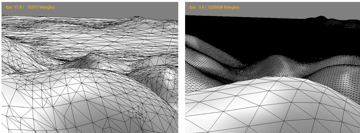
**Figure 9:** The Corresponding Wireframe: our implementation (left); Bézier patch implementation (right).
