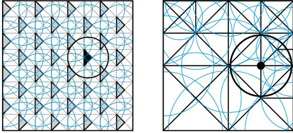
**Figure 2:** Local fitting of Bézier triangle patches from the method presented in <sup>19</sup> (left) compared to our BTT vertex fitting (right). The highlighted triangle and vertex are shown with their respective initialized local area circles. Meshes are shown at densities for sampling 320 data points with  $N_{\Delta} = 10$ .
