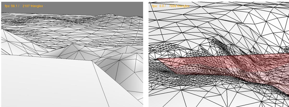
**Figure 10:** Our implementation without butterfly subdivision (left). Outside point of view of mesh tessellation (right).
