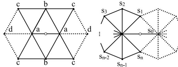
**Figure 4:** The modified butterfly scheme ten point stencil (left), and extraordinary vertex stencil (right). A new vertex is created at the position of the circle by the weighted sum of the stencil vertices. Weights  $a, \dots, d$  and  $s_0, \dots, s_n$  are specified in<sup>39</sup>.
