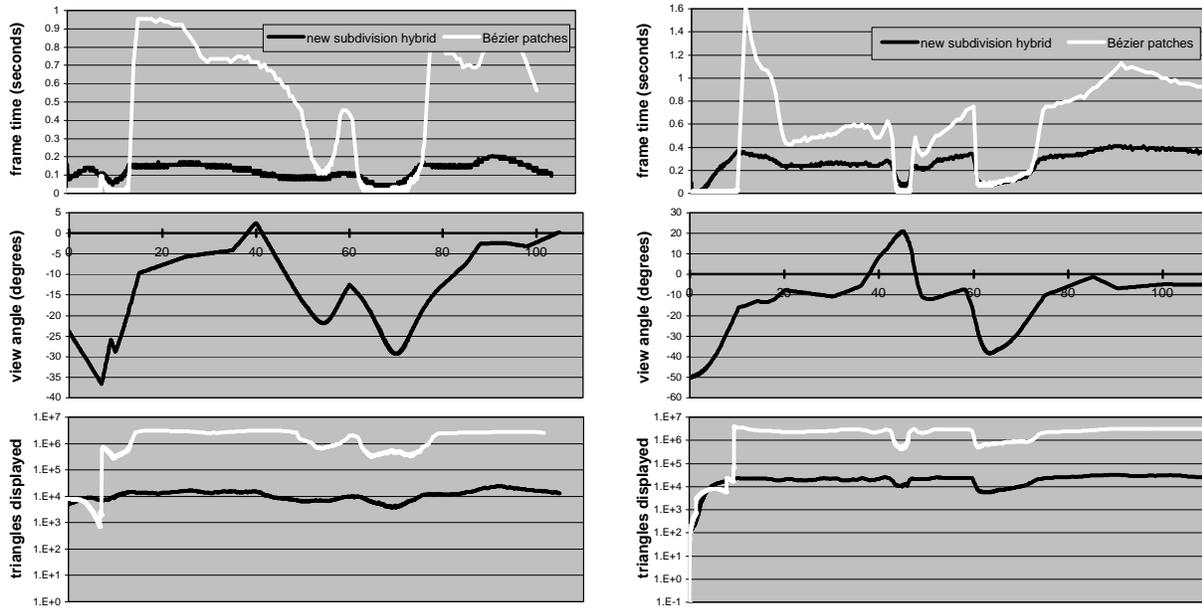
**Figure 7:** Frame computation times and triangle counts for two fly-through animations of the Dense and Fractal data sets (left and right, respectively). Our new implementation (black) is compared with the Bézier patch method<sup>19</sup>(white). Values are plotted over time in seconds of the animations. These are the same as seen in the accompanying videos. Note the strong impact viewing angle has upon the Bézier patch method.
