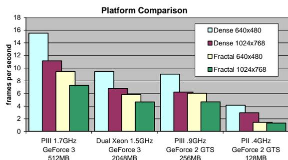
**Figure 6:** Average frames per second for two data sets and resolutions for scripted fly-through animations.
