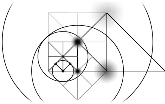
**Figure 5:** An illustration of nested circles in 2D on a BTT. Centers are marked by soft dots of increasing size higher in the tree. Not all BTT edges are shown, only edges connected to centers.
