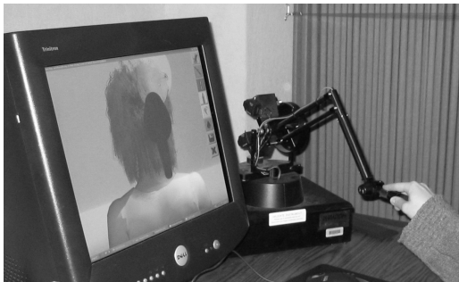
Figure 2: User Interface: PHANToM provides 3D user input and 2D menu buttons are labeled with icons to show applications.
