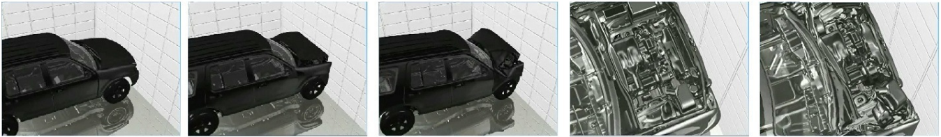
Figure 2: Sequence of simulation steps for the Car Crash benchmark with about 1.1-1.2 million triangles [Tang et al. 2011b]. We can reliably compute all collisions in about 15 seconds on a single core.
