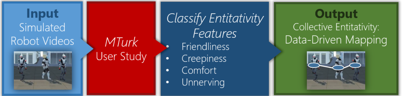
Fig. 3: We generate a variety of simulated robot groups using our motion model. Based on our precomputed EDM, we classify the entitativity of each cluster or group of pedestrians based on the four components: friendliness, creepiness, unnerving, and comfort.
