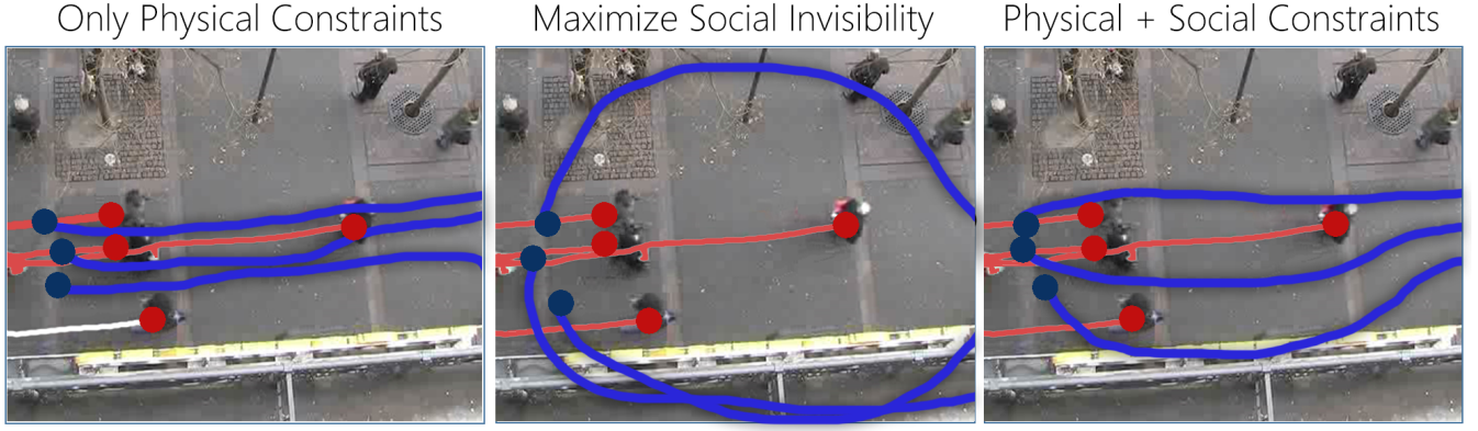
Fig. 5: Example robot trajectory navigating through the crowd in the Hotel dataset. Red circles/trajectories represent current pedestrian positions and blue circles/trajectories are the current positions of the robot. The left figure computes paths based on only physical constraints (collision-handling, smooth trajectory computation, sensor errors and uncertainty, and dynamics) at the cost of higher social constraints (zero social invisibility); the middle figure minimizes social constraints (i.e. entitativity) at the cost of longer paths; the right figure (our algorithm) balances social and physical constraints, and computes appropriate trajectories for the robot (in blue ).
