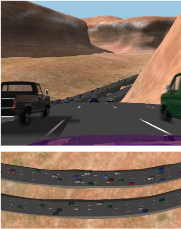
Fig. 1: Images of highway traffic synthesized by our method. Our method computes trajectories one by one for a continuous stream of cars (of possibly high-density). The trajectories fit the boundary conditions at the sensor points, and obey the geometric, kinematic and dynamic constraints on the cars. The number of lane changes and the total amount of (de-)acceleration are minimized and the distance to other cars is maximized to obtain smooth and plausible motions.
