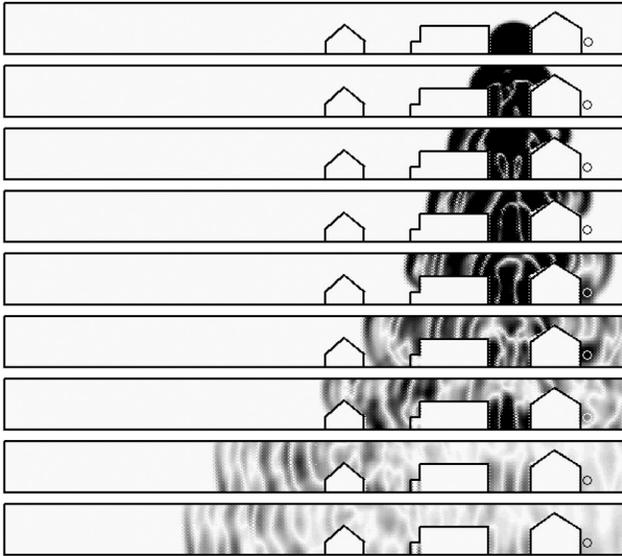
FIG. 12. Rooftop diffraction. Calculated acoustic response for the source position SP1 in the artificial village scene using the ARD technique. Receiver position R09 is marked by a circle on the side of the first building (from right). Simulated wavefields are shown at times  $t = 20, 30, 40, 50, 61, 83, 104, 161,$  and  $177$  ms corresponding to marked points in Fig. 10.
