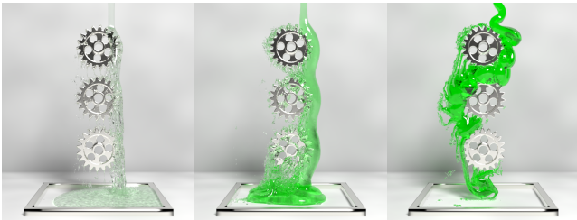
Figure 9: Three gears interacting with viscous fluids with \eta = 1.0 \times 10^1, 1.0 \times 10^2 and 1.0 \times 10^3 kg/(s·m) from left to right. Different viscosity values induce distinct fluid behaviors and solid rotations.
