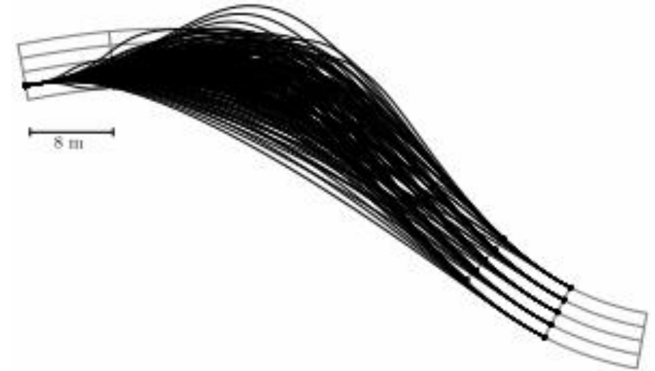
Fig. 5: State transitions on the transformed grid. The successors of one vertex are shown in black.
