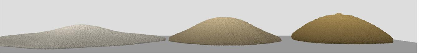
**Figure 4:** Three stable piles with friction coefficients  $\alpha = 0.3, 0.5,$  and  $0.7,$  respectively. Lower friction leads to flatter piles.
