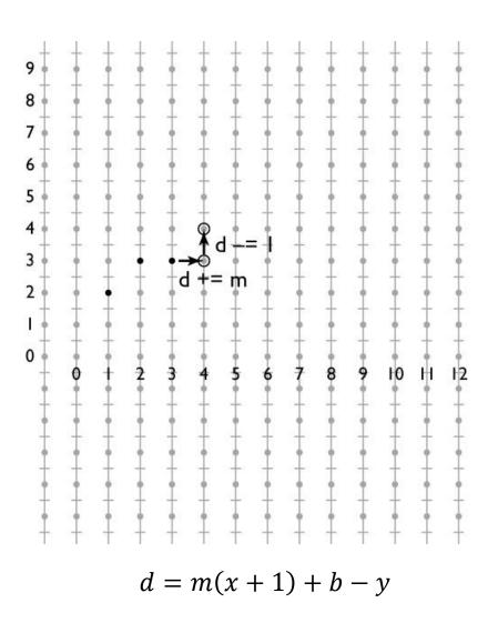
$\begin{array}{l} x = ceil(x_0) \\ y = round(m^*x + b) \\ d = m^*(x+1) + b - y \\ while x < floor(x_1) \\ if d > 0.5 \\ y += 1 \\ d -= 1 \\ end \\ x += 1 \\ d += m \\ mark(x, y) \\ end \end{array}$
