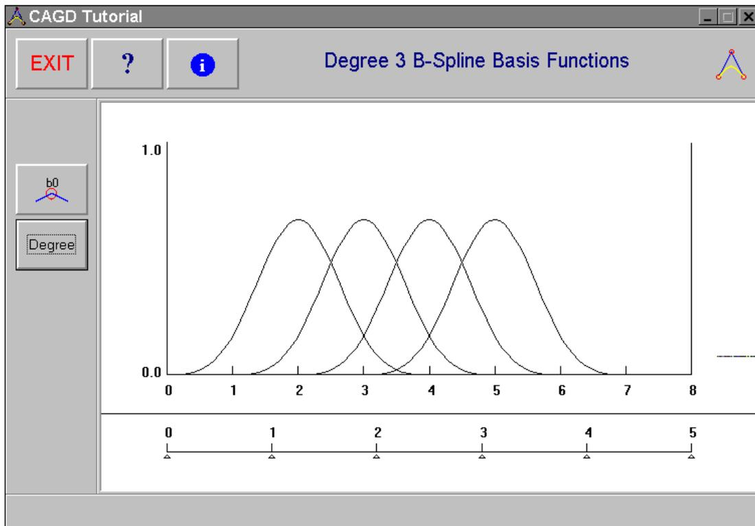
Here, the figure shows the cubic B-spline basis functions for a non-uniform knot sequence. The knot sequence is shown beneath the basis functions.
