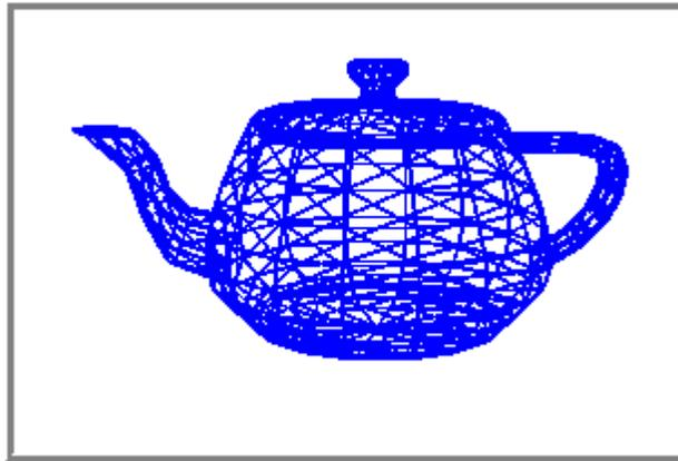
When the Bézier curves are created and connected in three dimensions, a wireframe model of the object is produced.
