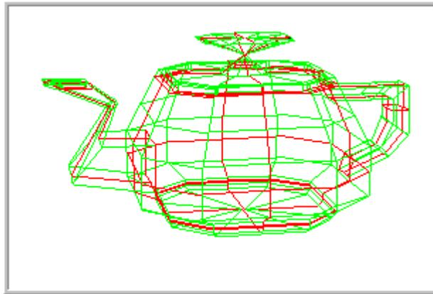
Bézier curves behave just as well in three dimensions as in two. This figure shows the control polygons for a three-dimensional object consisting of Bézier patches<sup>4</sup>.
