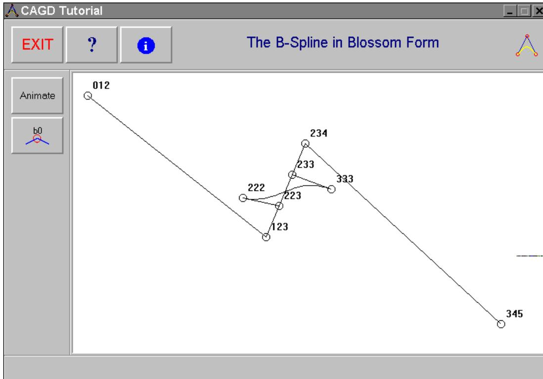
The additional points are computed with the EvalBlossomProg routine, which was introduced in the topic on blossoms. The new points **012**, **123**, **234**, and **345** are called the de Boor<sup>1</sup> points. When a curve is given by these points (instead of, for example, the Bézier control points), it is called a B-spline curve<sup>2</sup>.
