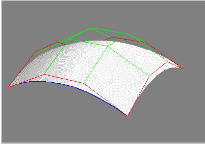
Each marginal set of control points defines a Bézier curve (the four border curves) and each of these curves is a boundary of the Bézier surface patch. Such a curve is shown at the forward edge of the patch in the picture above.
