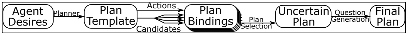
Figure 1: Two-stage Action Planning with Incomplete Information: Each agent is given a desire to achieve during simulation. We propose a two-stage planner which generates action plans despite uncertainties in the agent’s knowledge. The first stage generates a plan template and a set of candidates for each argument in the plan. The second stage generates a set of candidate bindings. The algorithm selects the plan with the least uncertainty and generates an action plan from the bindings. If any uncertain information is present, an uncertainty resolution action is created, yielding the final action plan which may include asking questions, or exploring the environment.
