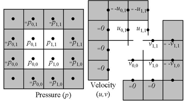
Figure 4: Setting Pressure And Velocity Boundary Conditions.
