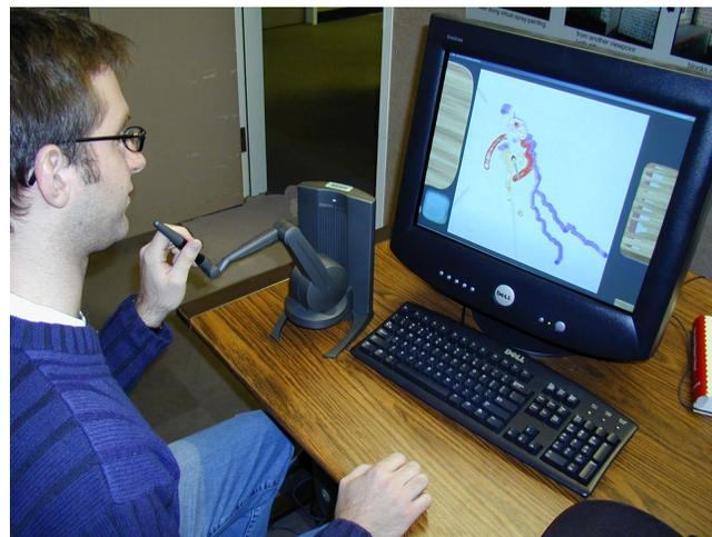
Figure 2: A Prototype Painting System Using PHaNTOM<sup>TM</sup> with the Graphical User Interface, the Virtual Canvas and the Brush Rack.
