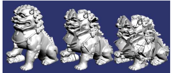
Figure 10: Benchmark Breaking Lion: In the benchmark, a lion model with 870K points has been crushed and is breaking into pieces. We compute the convex hull of the point set during each time step of this simulation.
