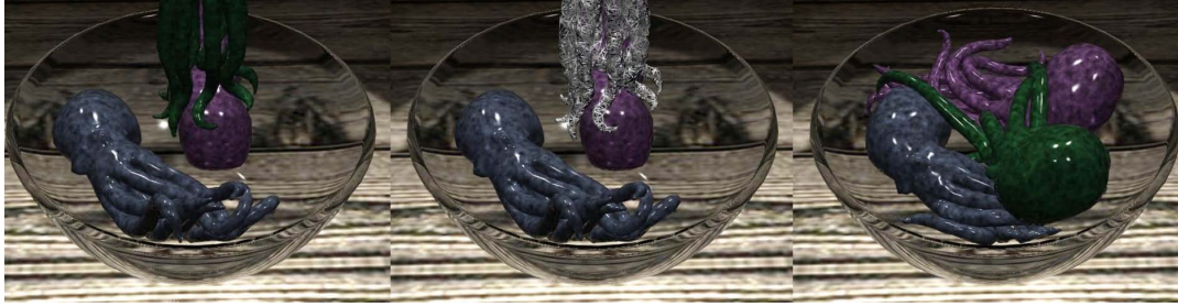
Fig. 7. Octopi Benchmark: Three deforming octopi with 24 tentacles consist of 17.6K tetrahedra. The simulation has multiple inter-object and intra-object collisions. The average CCD query time is 75ms per frame.
