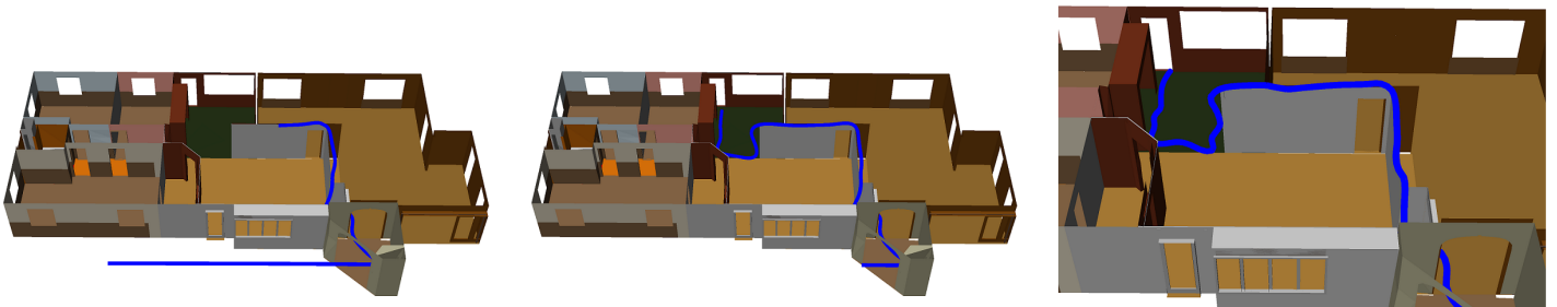
Figure 8: Cable route planning on the House Model
