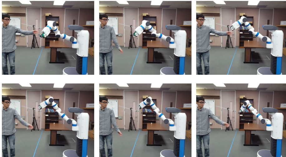
Fig. 5: Real Robot Experiment: We evaluate our planning algorithm on 7-DOF Fetch robot arm to compute collision-free robot motion. Our bounded probabilistic collision checking is used for computing safe trajectories.
