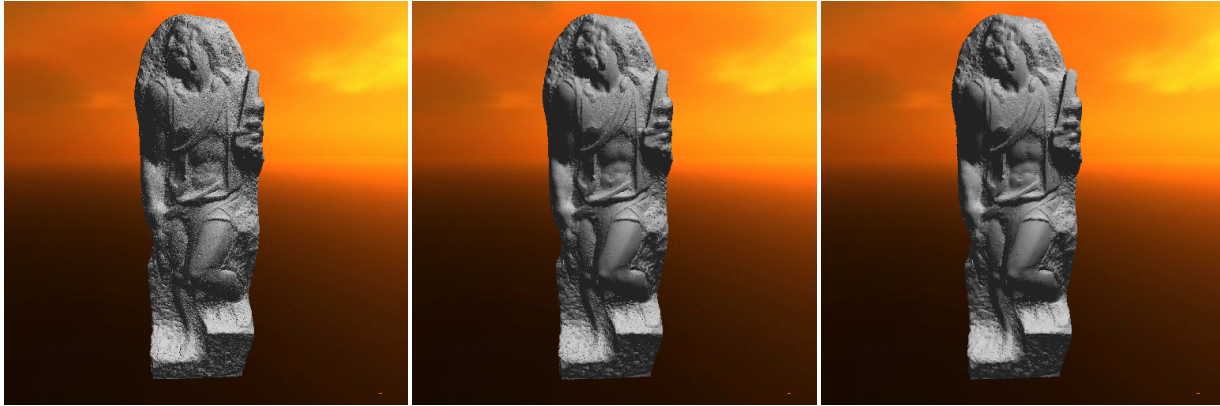
Fig. 8 Images of the St. Matthew model with different PoE values are shown at 512 \times 512 image resolutions. We do not use anti-aliasing to highlight image quality difference. Please note that the original St. Matthew model has many holes. The use of R-LODs can alleviate aliasing artifacts and improve the performance of massive models.
