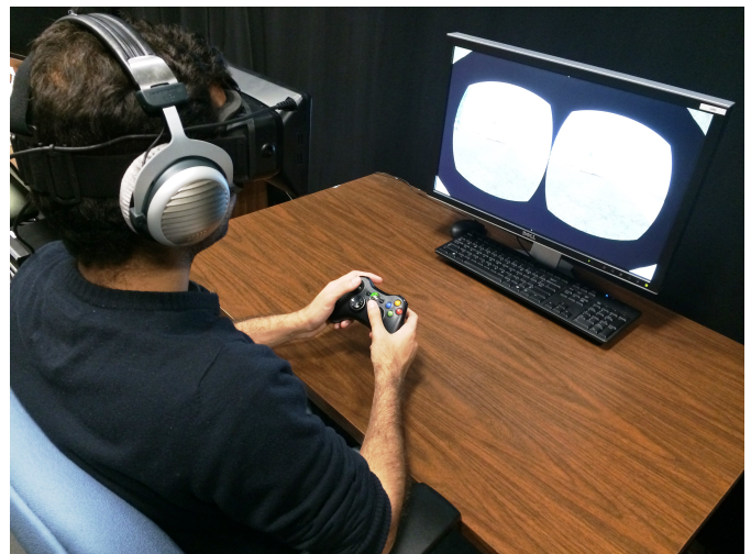
Fig. 1. User experiencing a VR environment with our WAVE sound propagation system. Our system tracks player’s interactions using the Oculus Rift head-mounted display (HMD) and the Xbox 360 controller and delivers high-fidelity acoustics effects and spatial sound using headphones.
