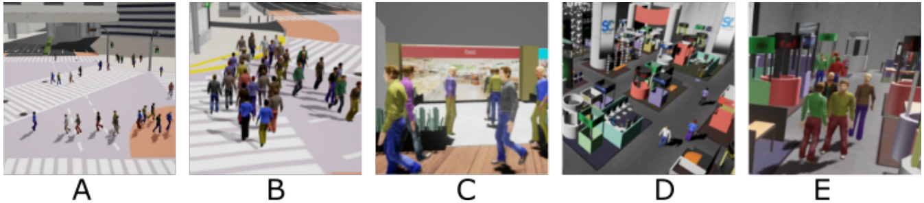
Figure 1: Our full-body crowd simulation algorithm generates smooth and natural-looking collision-free trajectories for multiple agents at interactive rates using a coupled 2D planner and full-body motion synthesis. (A) A busy city crossing with multiple agents. (B) Agents show natural crowd behaviors such as lane formation. (C) A shopping mall scenario where agents pass each other in narrow hallways and walk up to shops. (D) A tradeshow scene where agents can be seen smoothly avoiding each other in narrow passages, and (E) even sidestepping in dense situations. Our algorithm can simulate and render 30 agents at 30-35 fps.
