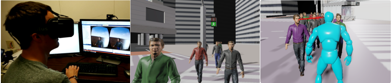
Figure 1: Our algorithm generates plausible full body motion for tens of virtual agents and allows the user to interact with the virtual crowd. (Left) The user is provided with a first person view through an HMD. (Center) The virtual characters display plausible behaviors such as gazing and gesturing. (Right) The real user (shown in blue) can freely move in the virtual world while the agents actively avoid collisions. We highlight the gaze using line-of-sight between real user and a virtual user.
